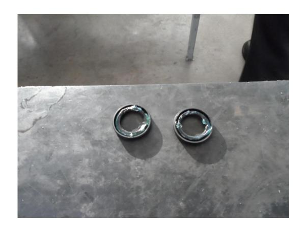
19) Place oil lip onto crank (Vaseline side inwards) and using a socket head and force of hand, push. Repeat on other side.
