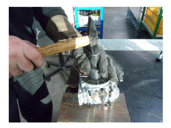
15) The crank should move freely within block.
