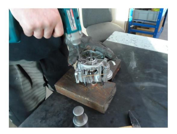
13) Use torque wrench to tighten. Minimum 12 Nm but we use 14 Nm  $\,$
