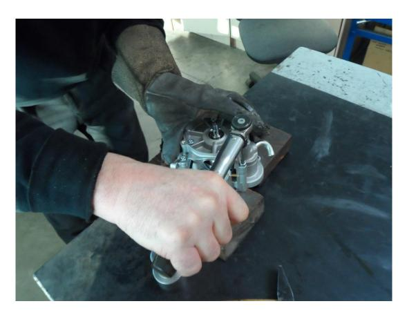
14) Using tool or perhaps a tall socket head, tap with hammer around the crank. You must NOT touch the protruding crank.
