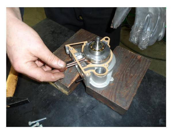
10) Check so other half of block has a temperature of 80°C and lower onto prepared first half of the block
