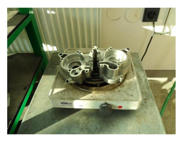
8) When temperature reaches 80°C remove one halve and place on wooden blocks and place crank inside
