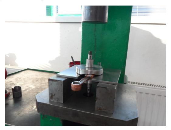
5) Place ball bearing onto crank and place round tool (possible to use socket heads) and press.
