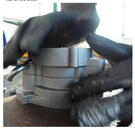
11) Press the spring pin through the blocks first
