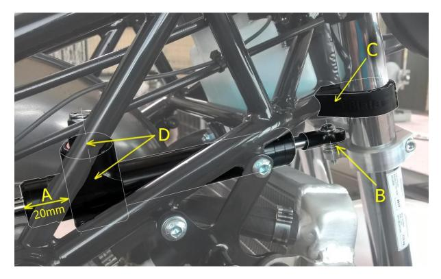
Correct mounting of steering damper so as to prevent hard impacts and bending of bracket on frame during extreme steering positions.
